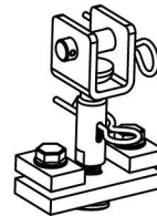
75 Crane Suspension Eye
