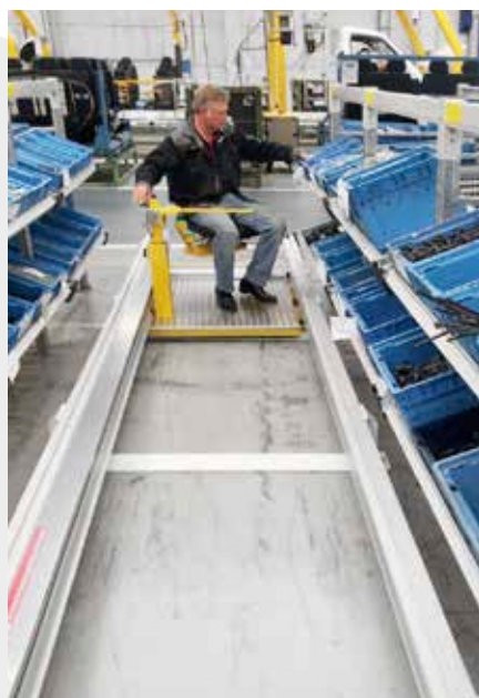
Guide rail installed in the floor or floor-guided lifting units
